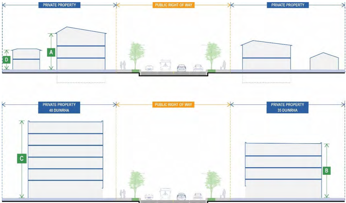
Figure 13.4: Building Profile Standards – Building Height
